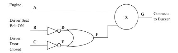
Copy and complete the truth table below, including the values produced by the unknown logic gate  $\mathbf{X}$ .
