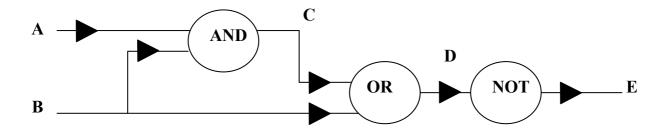
Complete the truth table for the four possible inputs A and B.
